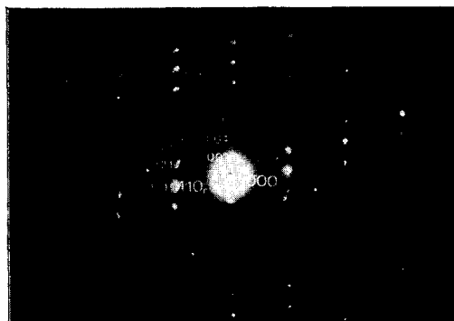
FIG. 1. Diffraction pattern of Cr_6O_{11} , a member of the (1\bar{2}1) family of CS structures in CrO_2 . Zone axis [1\bar{1}\bar{3}]_r . The indices to the right of any vertical row—subindexed r —belong to the basic rutile-like cell, the indices to the left belong to the Cr_6O_{11} cell.
